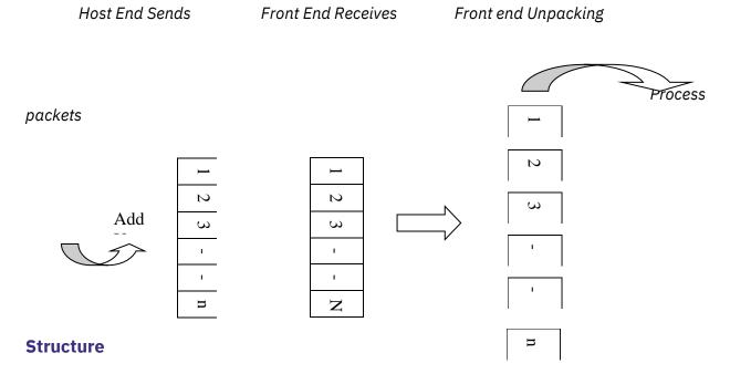
Incoming packet at the front end can be interpreted by mapping onto the following structure.
