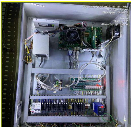
Figure 3-9: Toll Lane Controller at Tunnel
