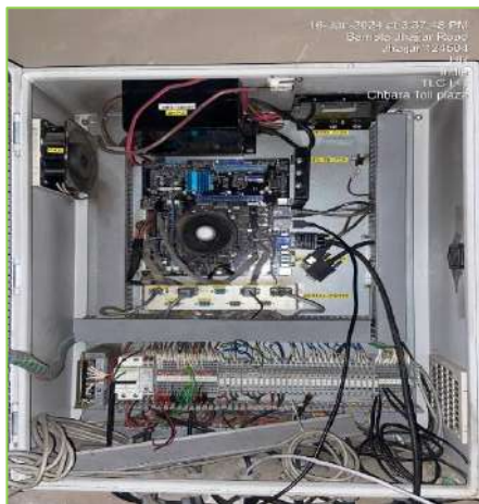
Figure 3-10: Toll Lane Controller at Tunnel
