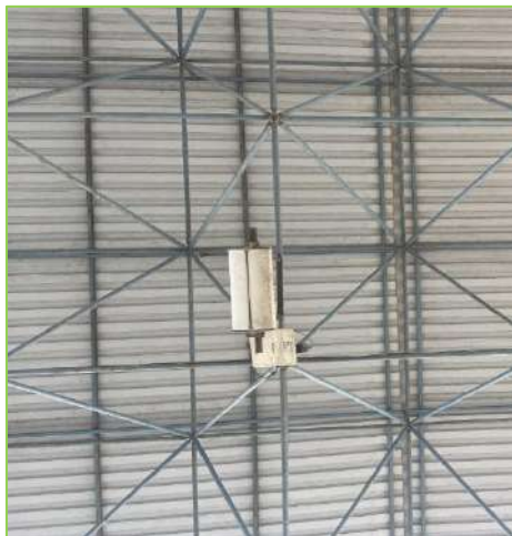
Figure 3-9: RFID reader.
