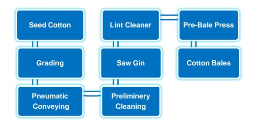
The main operation of separating seed from cotton is done by saw gin. In the gin house after ginning process is completed the cotton lint and cotton seeds are separated and the lint passes out through pneumatic system to the Post-cleaner (Lint Cleaners) in which small impurities, dust particles, small fibers are carried out and cotton becomes free from contamination.
