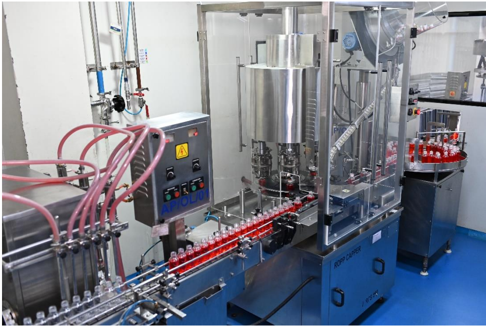
Liquid Filing and Sealing
