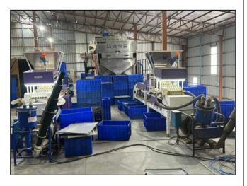
The cashew kernel sorting process employs color Sortex and size Sortex machines to enhance quality and consistency. The color Sortex machine separates kernels by color, ensuring uniformity and removing discolored or defective pieces. The size Sortex machine categorizes kernels by size, meeting market requirements and optimizing packaging and distribution efficiency. This process enables the delivery of cashew kernels that meet quality and market standards
