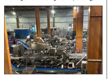
The cutting of raw cashew nuts (RCN) in our shelling machine is an operation essential for extracting kernels efficiently and minimizing waste. Our advanced shelling machines are configured to carefully crack open each nut, separating the shell from the kernel with precision. This process ensures maximum yield and maintains the integrity of the kernels, meeting our commitment to quality and efficiency in cashew nut processing.
