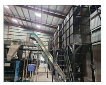
Our cooling facilities for raw cashew nuts (RCN) are designed to maintain optimal conditions after boiling. Post-boiling, RCN undergo controlled cooling to reduce moisture and oil content, which helps preserve freshness and quality. This controlled cooling process also facilitates the subsequent shelling step which prevents the spillage of oil during shelling, which may reduce the quality of the nuts.
