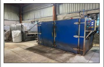
The NW (Natural Wholes) obtained after shelling, are dryed in the drying facilities, to reduce the oil content from the NW, so that the bitter taste of the kernels can be removed and further it ease the stickiness of the husk of it, which makes it easier for next step viz Peeling.
