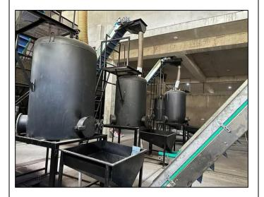
Steaming and boiling raw cashew nuts is a critical step in our processing, aimed at achieving optimal kernel extraction and quality. We control steam and boiling times to soften shells, facilitating kernel extraction while maintaining their nutritional content and natural flavor. Our precise steaming and boiling processes ensure that each batch meets our stringent quality standards, resulting in superior raw cashew nut products ready for further processing or distribution.
