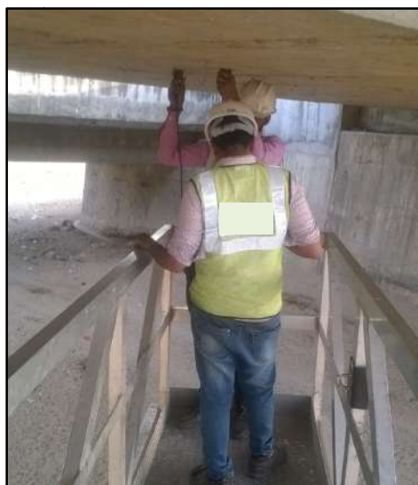
Figure 89. Operators conducting ultrasonic pulse velocity test
