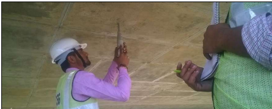
Figure 91. Operators conducting rebound hammer test
