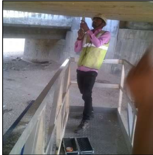
Figure 88. Operators conducting rebound hammer test
