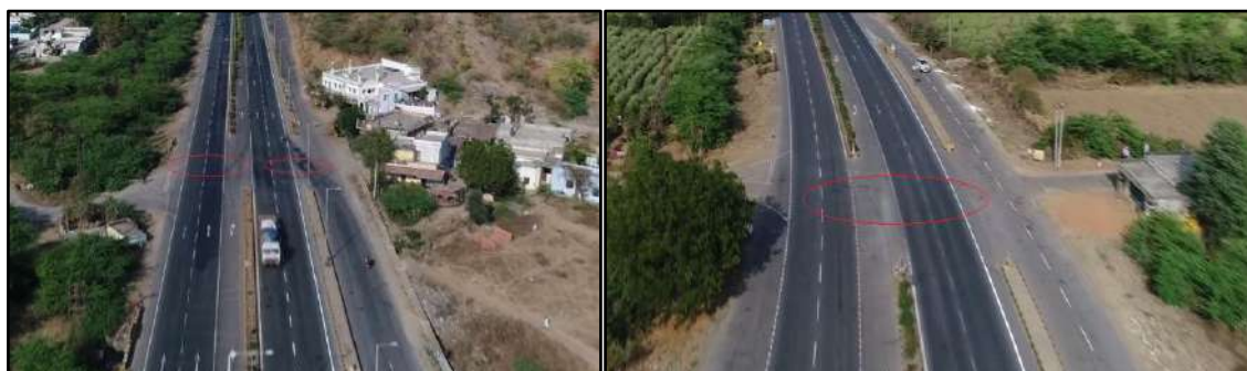
Figure 127. Photographs of Improper Pedestrian Crossing (647+050 and 657+300 respect.)
