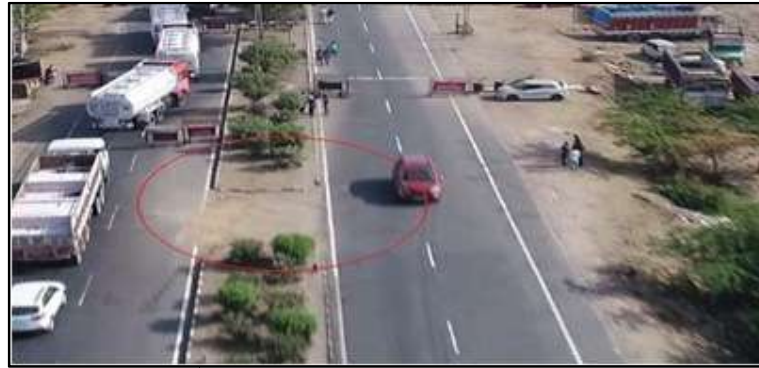
Figure 124. Photograph of improper medians cuts at 634+200
