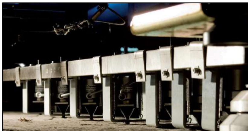
Figure 25. Falling Weight Deflectometer geophones
