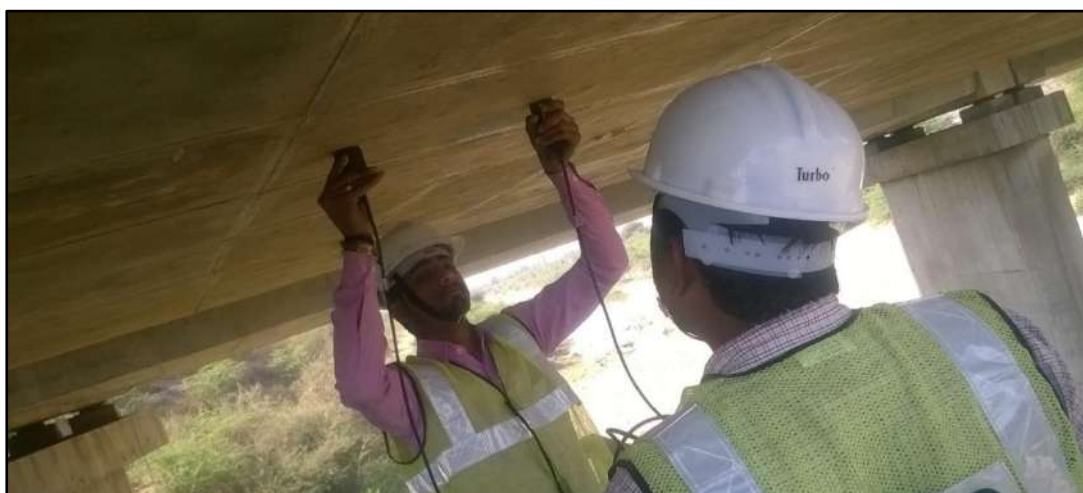
Figure 92. Operators conducting ultrasonic pulse velocity test
