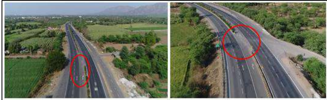
Figure 123. Pictures of improper medians cuts. 652+800 and 657+300
