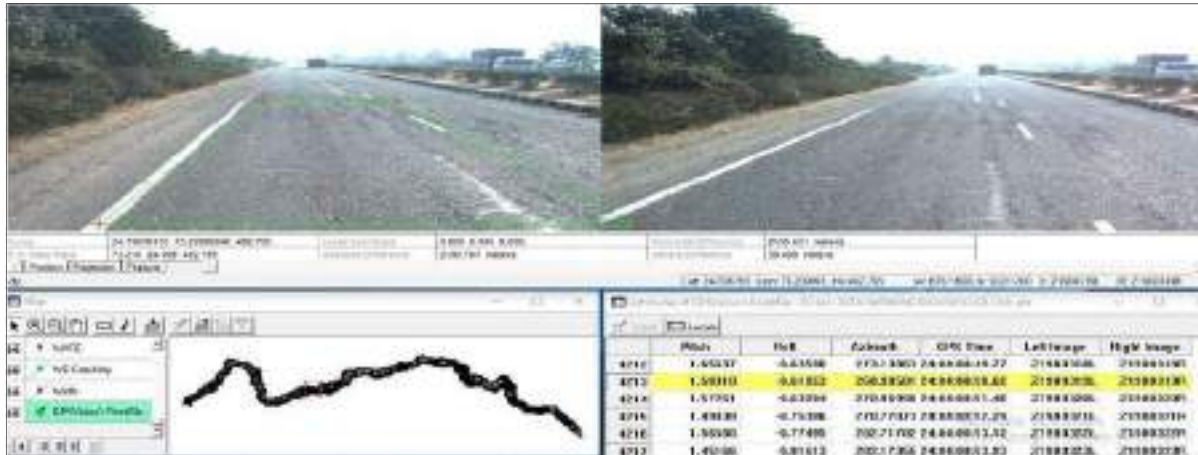
Figure 10. Snapshot of feature extraction of cracking
