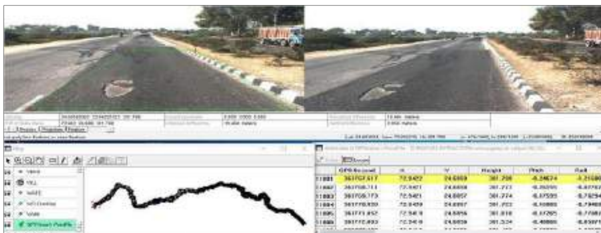
Figure 7. Snapshot of feature extraction of pot holes
