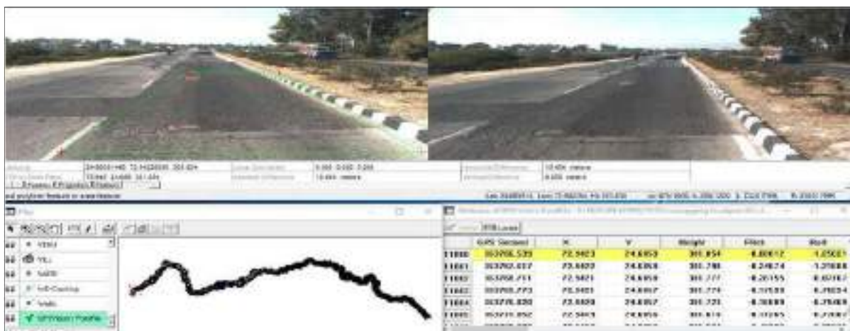
Figure 6. Snapshot of feature extraction of pot holes
