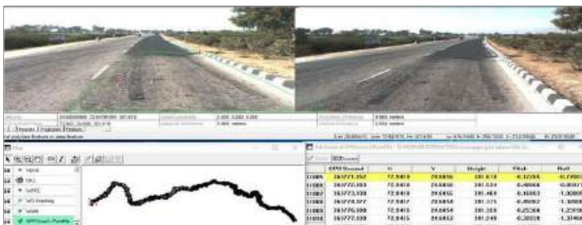
Figure 9. Snapshot of feature extraction of cracking
