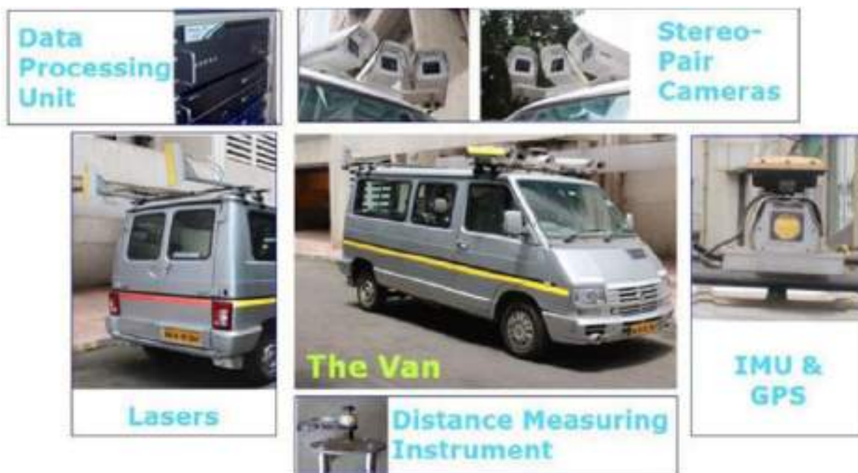
Figure 2 GPS vision system components
