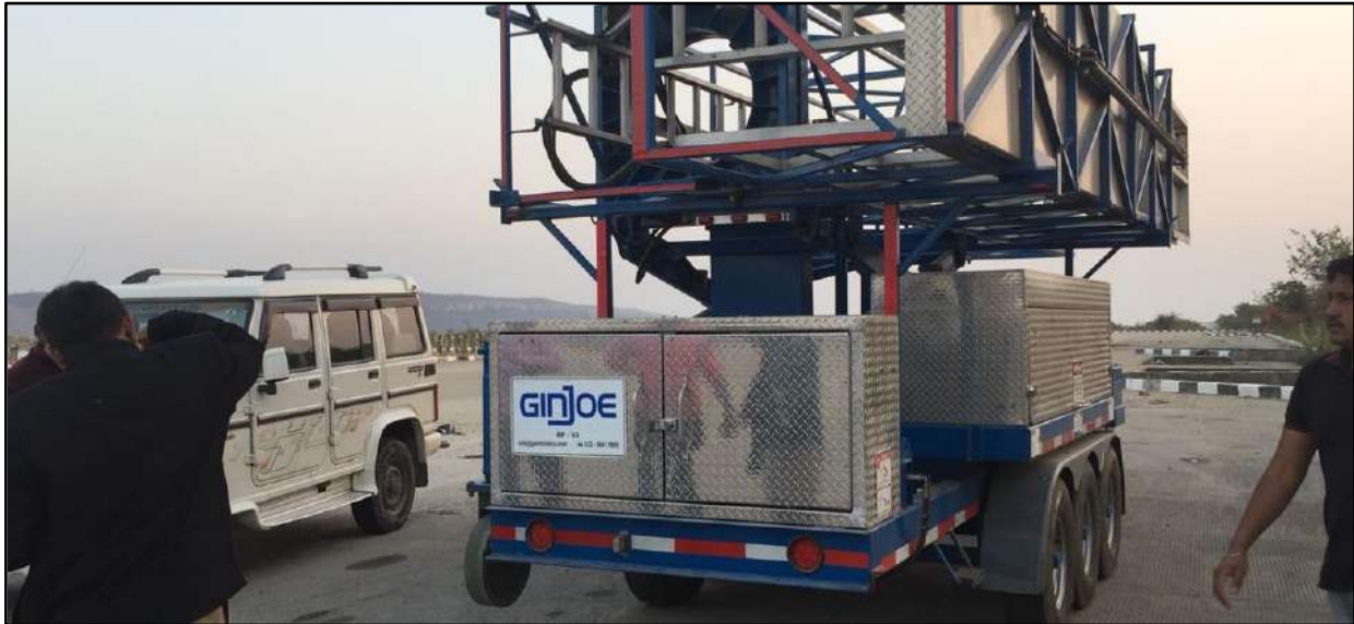
Figure 90. Mobile Bridge Inspection Unit used in inspections
