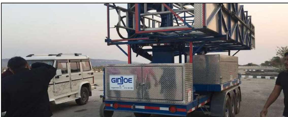
Figure 87. Mobile Bridge Inspection Unit used in inspections (MBIU)
