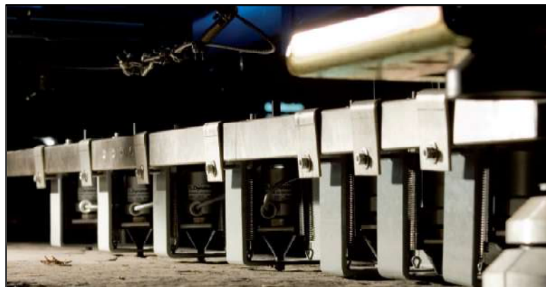
Figure 22. Falling Weight Deflectometer geophones
