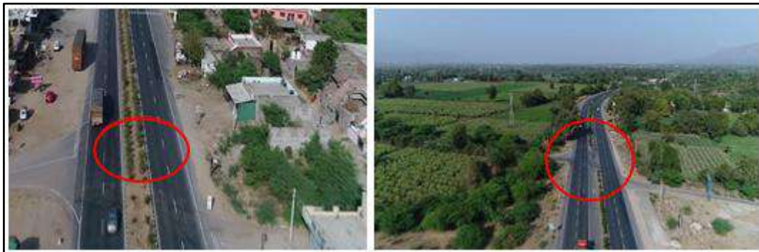
Figure 124. Pictures of improper medians cuts. 649+100 and 649+600
