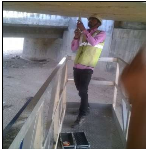
Figure 88. Operators conducting rebound hammer test
