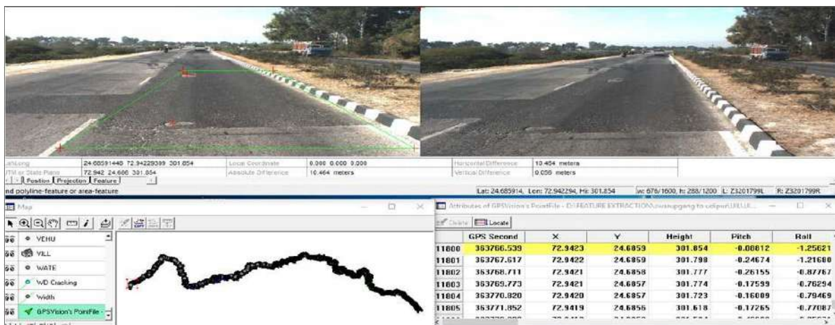
Figure 6. Snapshot of feature extraction of potholes
