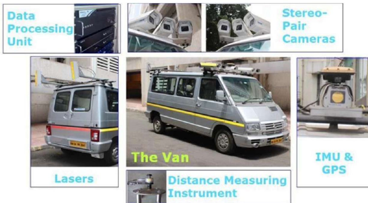
Figure 2: GPS Vision System Components
