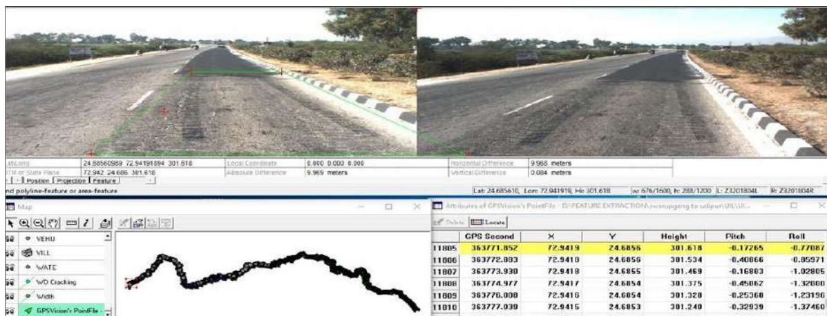
Figure 9. Snapshot of feature extraction of cracking
