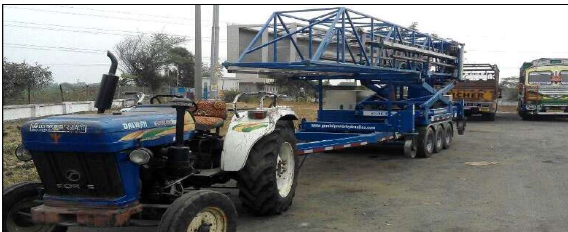
Figure 86. Mobile Bridge Inspection Unit used in inspections
