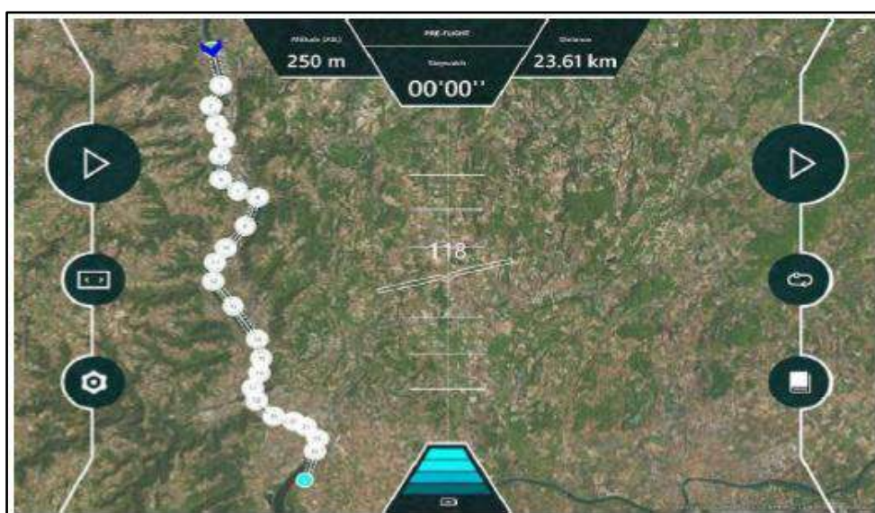
Figure 144. Sample of Software of Flight Planification
