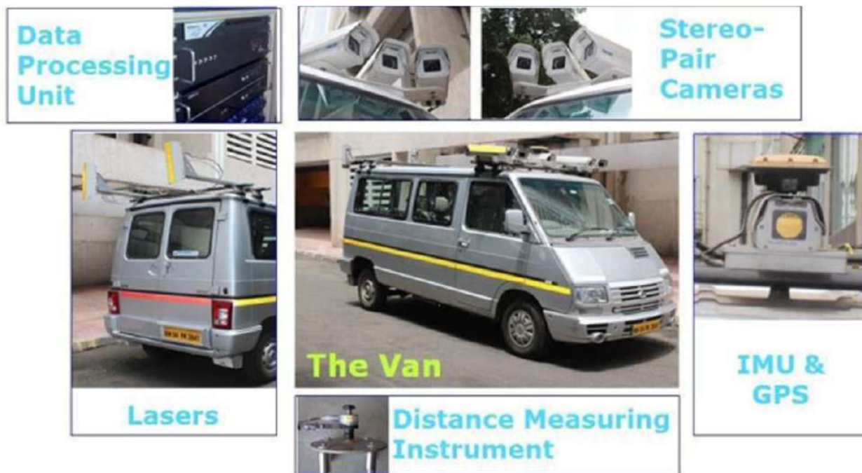
Figure 2 GPS vision system components
