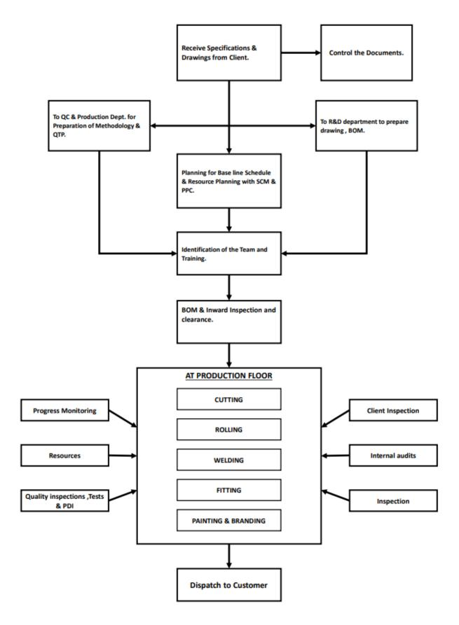
1. Receive Specifications & Drawings from Client: This initial step involves obtaining the necessary specifications and drawings from the client. These documents provide the essential details about the product requirements. Accurate and clear specifications and drawings are crucial for ensuring that the final product meets the client's expectations.
