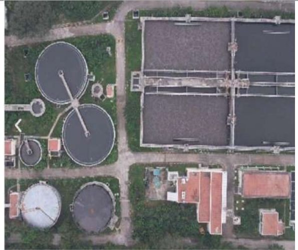
50MLD capacity Sewage Treatment Plant at Nesapakkam, Chennai with Sequential Batch Reactor (SBR) with Power Generation from bio-gas
