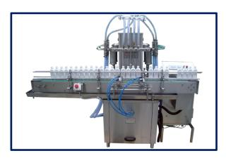
A liquid filling machine is a type of packaging equipment used to accurately fill containers with liquid products. These machines are commonly used in nutraceuticals products.
