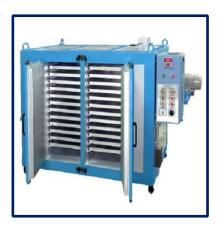
A tray dryer is a type of drying equipment used to remove moisture from solid materials or products. It typically consists of a cabinet or chamber containing multiple trays or shelves on which the material to be dried is placed.
