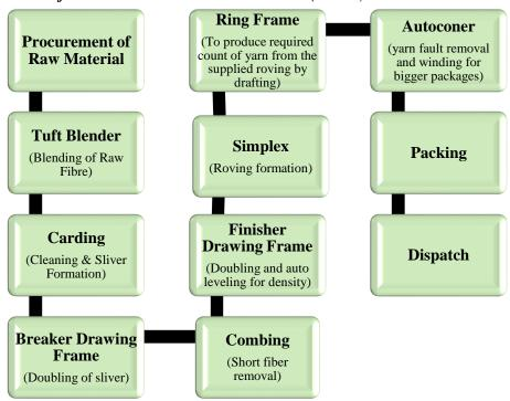
**Tuft Blender -** it is used to blend different types of fibers to create a homogeneous material with a uniform appearance. Tuft blending is particularly useful for ring yarns because it improves the homogeneity of the yarn, which is less blended on a ring spinning machine
