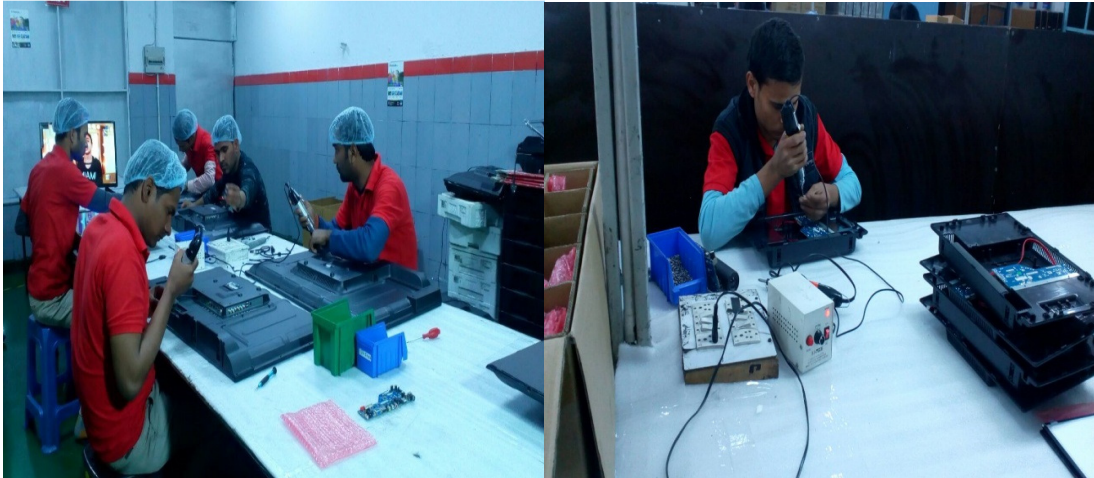
Assembling of LED TVs
