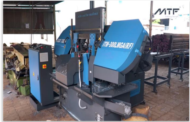
CNC Machine used for raw material cutting
