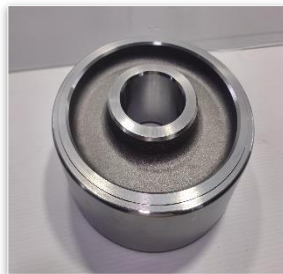
Gear component after machining stage.
