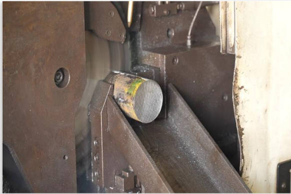
CNC Machine used for raw material cutting
