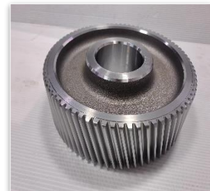
Gear component after teeth cutting process.
