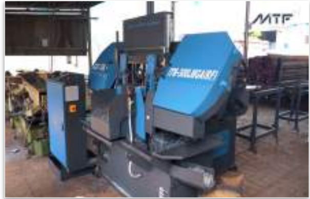
CNC Machine used for raw material cutting
