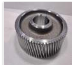
Gear component after teeth cutting process.
