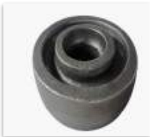
Gear component after forging stage.
