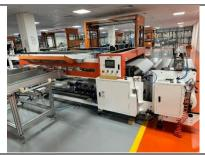
**EVA Cutting Machine** - Auto feeding EVA coiled material, auto cutting and punching, and laying it on the glass.
