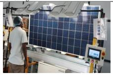
**90° Inspection -** Flip the modules to an angle that is convenient for manual observation to check the quality of the modules.
