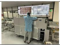
**Laminator** - It is used to join all the layers forming the module, ensuring immunity to the cell against dust, moisture, humidity, and other environmental conditions.
