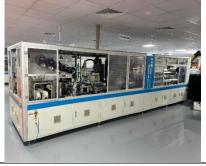
**Stringer-** Soldering equipment for serial connection between cells, Compatible with 5BB-9BB, 156-158.75 mm cells.
