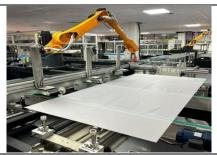
Layup Machine - Automatic Lay-up Machine adopts automation technologies such as PLC, servo, mechanical visual etc. Achieving solar string automatic laying on glass EVA and transporting module to the next process.
