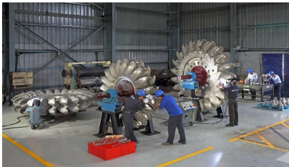
Rebuilding and refurbish of Pelton runner of Hydro turbine at our work
