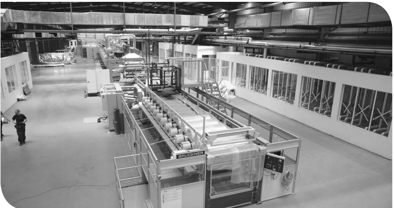
Max Speciality Films' latest production line (Line 5) is a five-layer line with inbuilt capability to produce thicker films with seamless speed.
