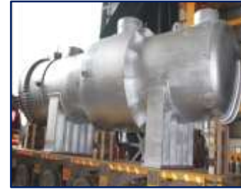
Moderator Heat Exchanger Used in nuclear island cooling systems
