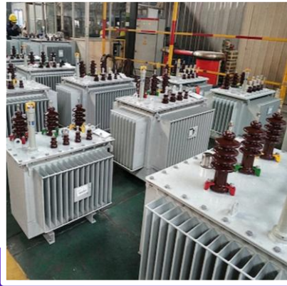
Manufacturing Of Distribution Transformers.
