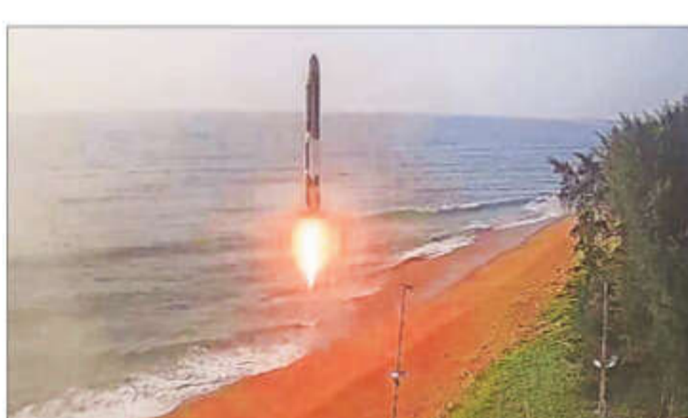
Agnibaan is powered by the world's first single piece 3D printed semi-cryogenic engine, according to Agnikul
