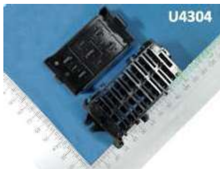
Fuse Box (14 Packs)
