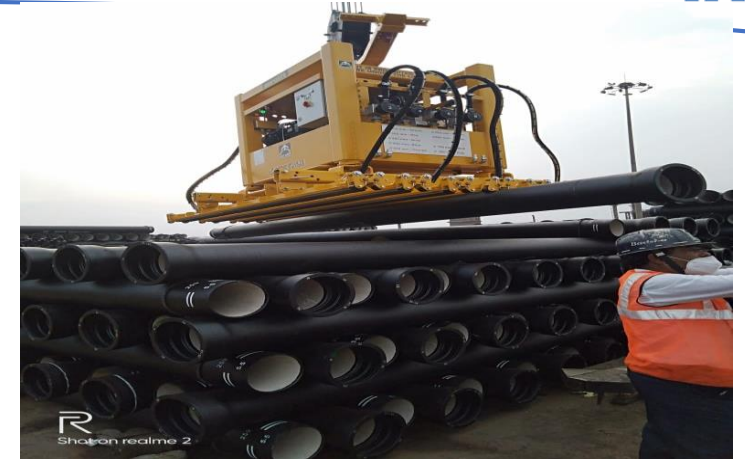
Vacuum Loading System for safe loading and despatch of Ductile Iron Pipes
