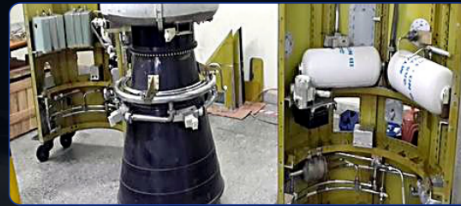
Agni A1 and A2 missile base shroud integration
