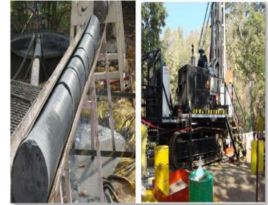
Large Diameter Kimberlite core (8") for Rio Tinto at Bunder, MP – Drilled by BLY LF230 upto a depth of 352 Meters. Largest coring done in India till date
