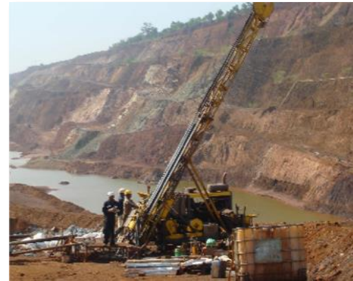
Core drilling for Chromite for Tata Steel Limited
