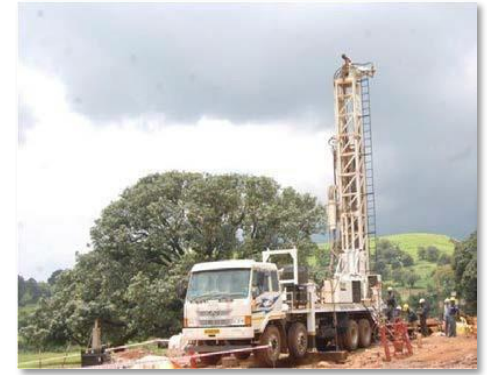
CBM Exploratory Drilling at Satpura, MP for Dart Energy
