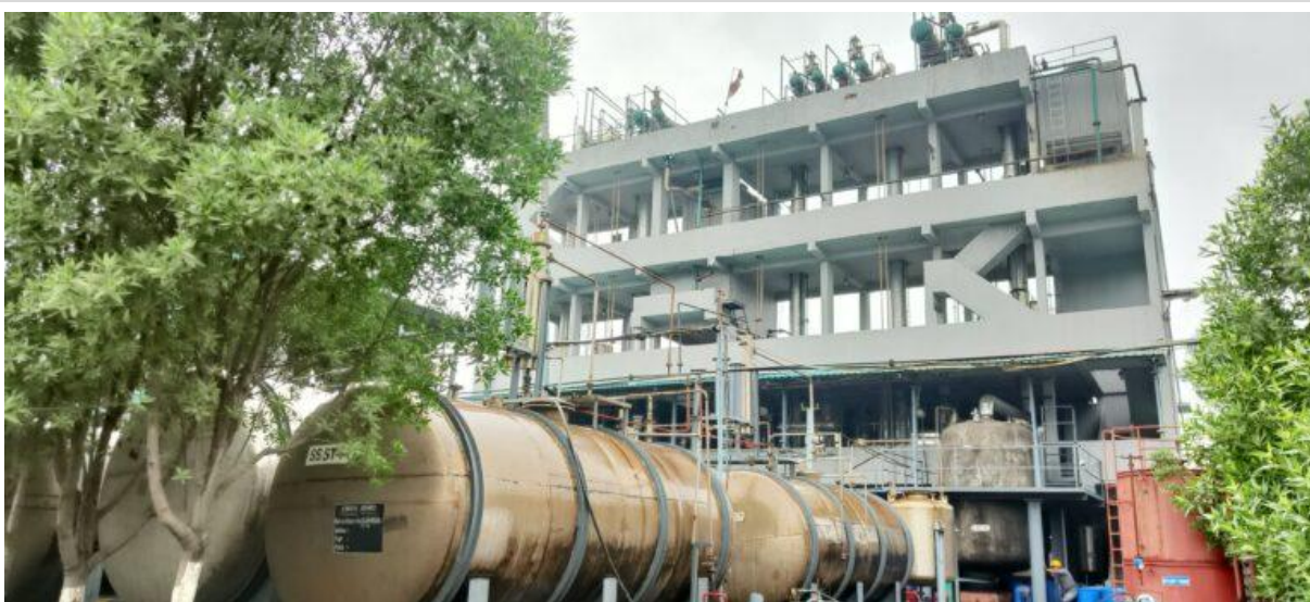
Multi-stage fractionating distillation and reactor unit used in the solvent recovery process.
