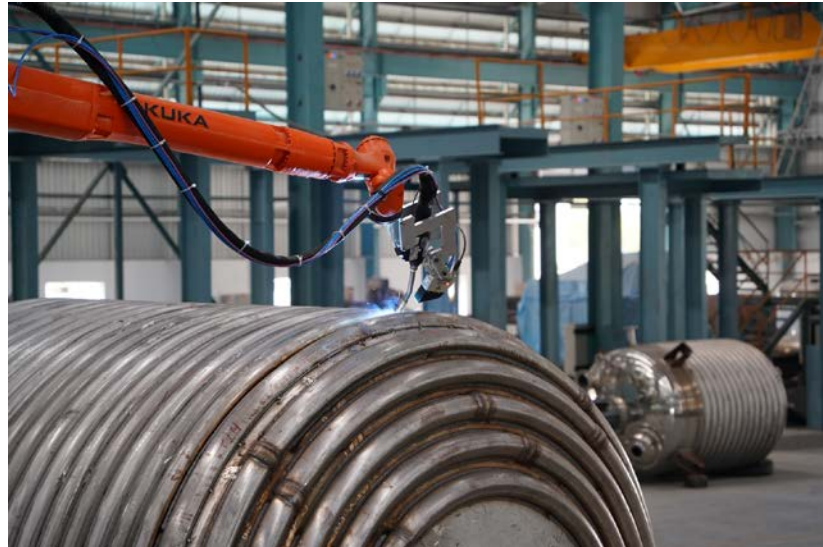
Robo welding process
