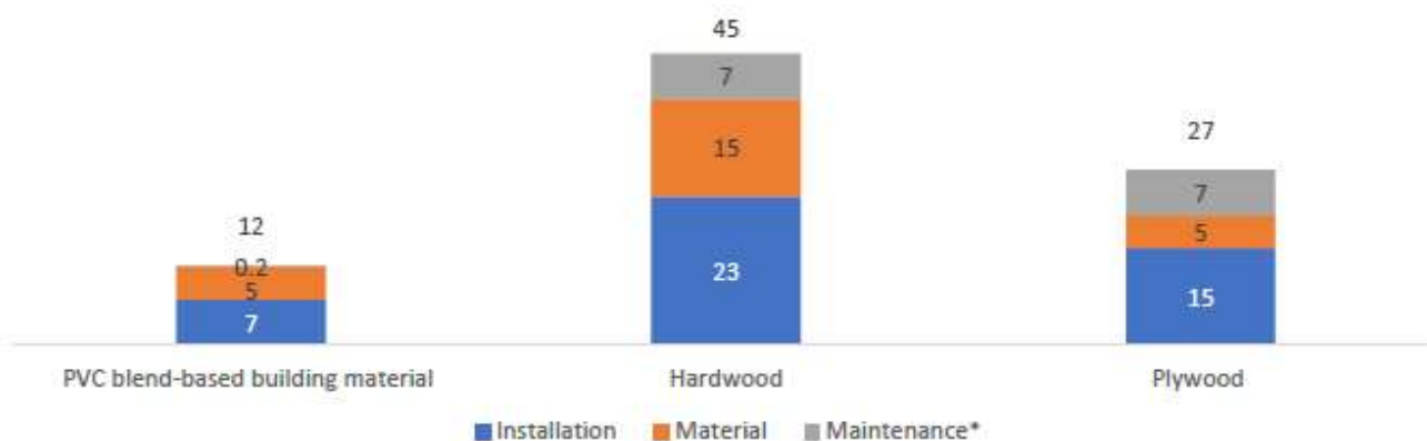
Figure 20: Life cycle cost of of PVC blend-based building material vs peers in flooring segment (US$/sq.ft)
