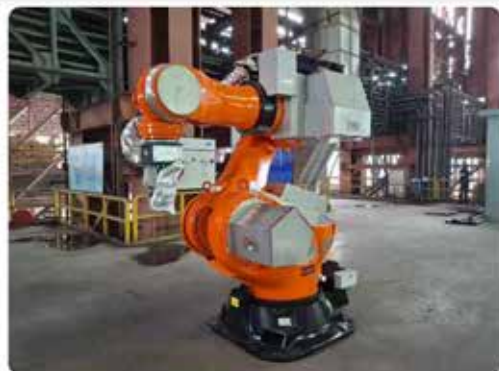
The automation reduces human exposure to molten metal, heat, and fumes while improving efficiency and product quality.
