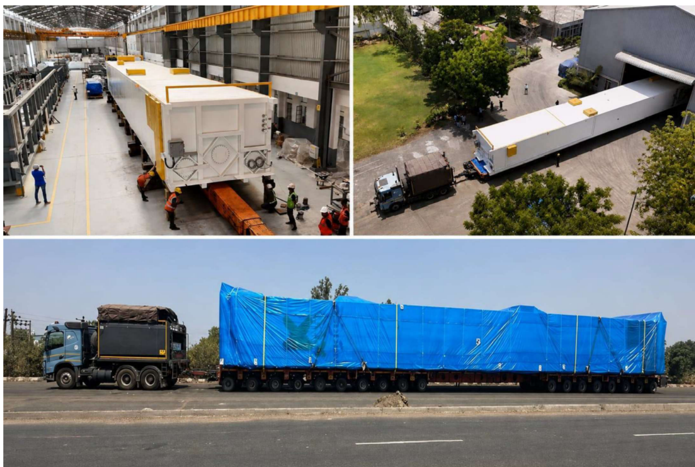
127-tonne, 127-foot cold box in transit from Baroda to Tirunelveli
