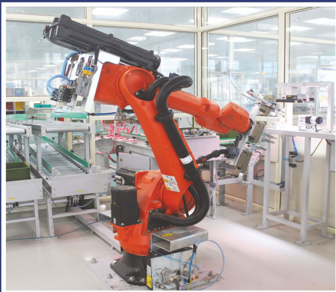
Robotic Marking Station for end to end process traceability
