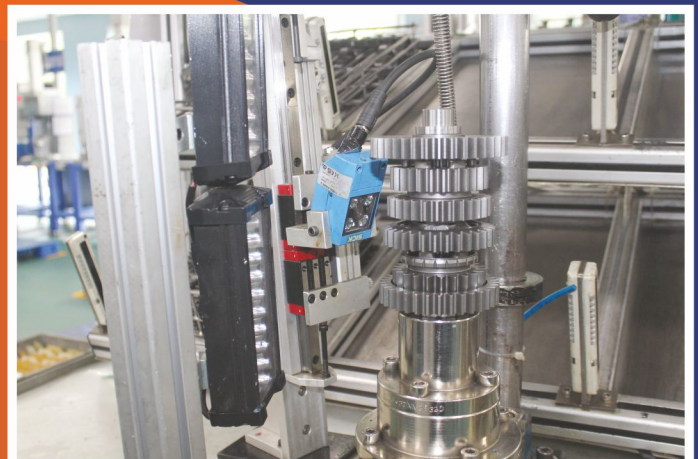
Assembly Station with camera based 100% mistakes proofing solution
