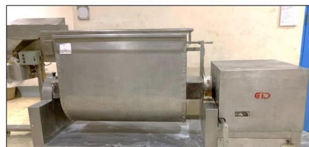
Mass Mixer Machine use for Powder Mixer
