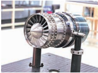
The short-duration turbojet engine can power tactical cruise missiles, anti-ship missiles, and loitering munitions
