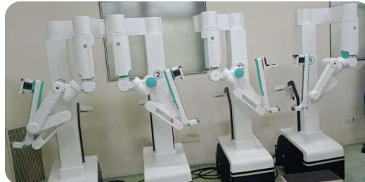
Robotic arms equipped with 3-D imaging
