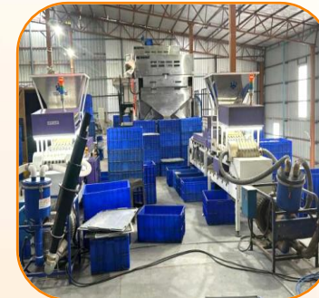
Sorting the Kernels Using Colour Sortex & Size Sortex
