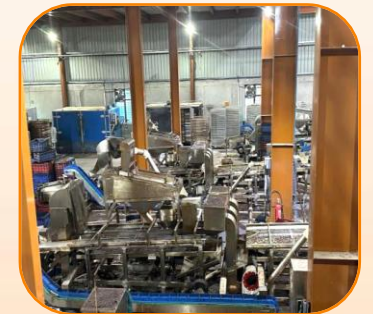
Cutting of RCN in Shelling Machine (Deshelling)
