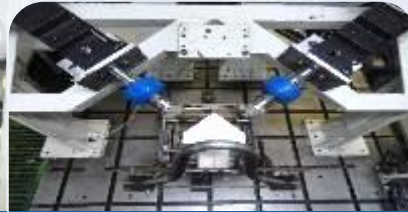
Right & Left Back 45 deg Moment Durability Test
