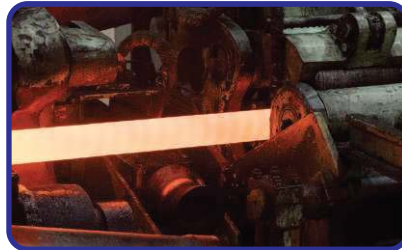
Hot Piercing Facility
