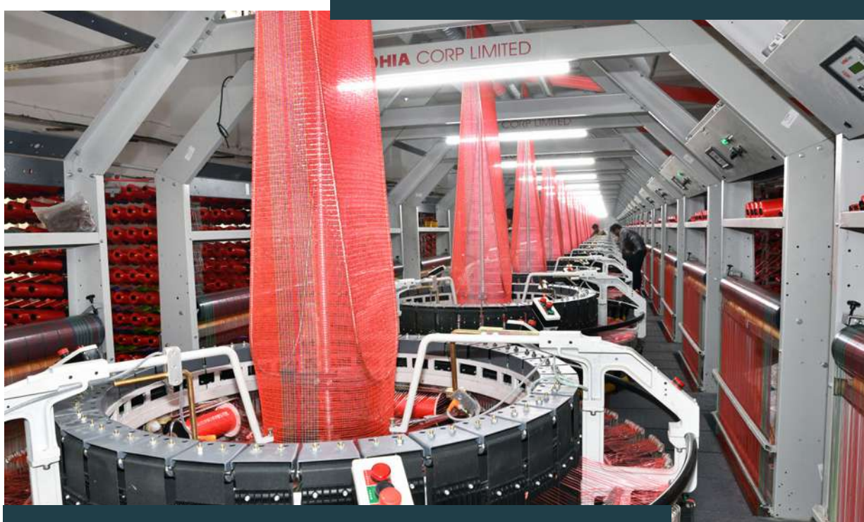
Automated circular looms efficiently weave high-strength leno bags for agricultural packaging.
