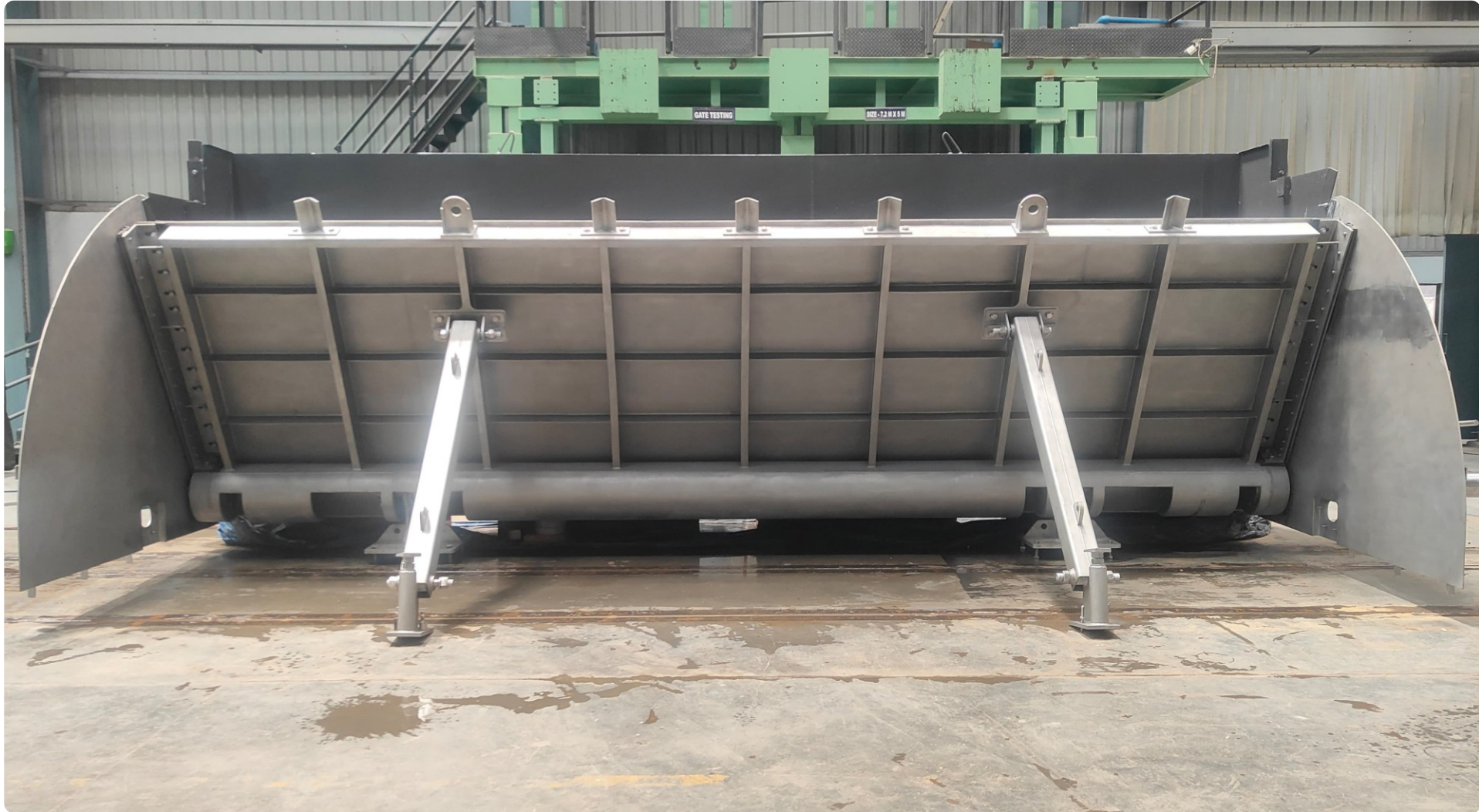
Stainless steel crest gate, 25' (7620 mm) X 5'-6" (1675 mm) – 1 No.
