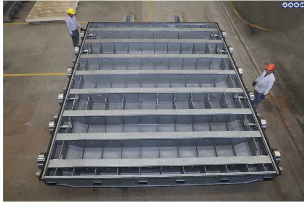
5250 mm X 6550 mm and 3275 mm X 6550 mm Roller Gates
