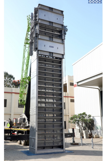
2500 mm (W) X 12,975 mm (H) Travelling Band Screen
