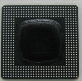
500 ball TBGA, 3 Tier wire bonding
