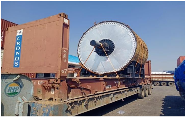
Flat Track on Container Vessel, Weight: 45 Metric Tons each, Length: 5-meter, Width: 4.33-meter, Height: 4.9 meter
