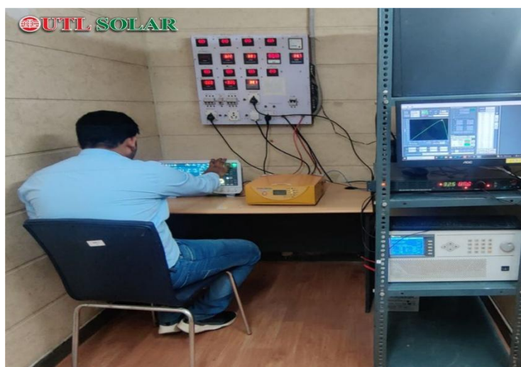
Off grid inverter testing set up
