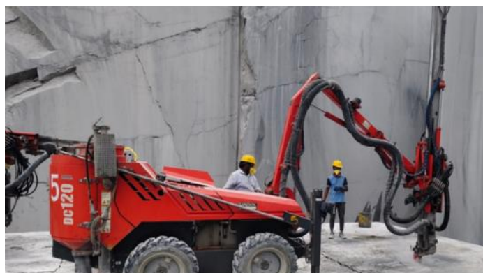
Drill machine equipped with dust sucking mechanism
