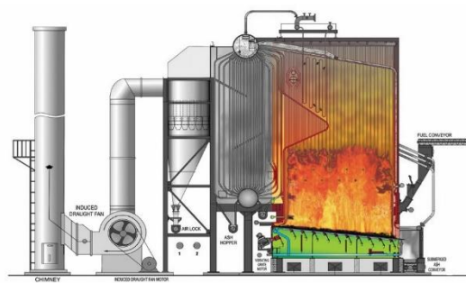
Exhibit 3.13: Process diagram of a biomass boiler based steam generation
