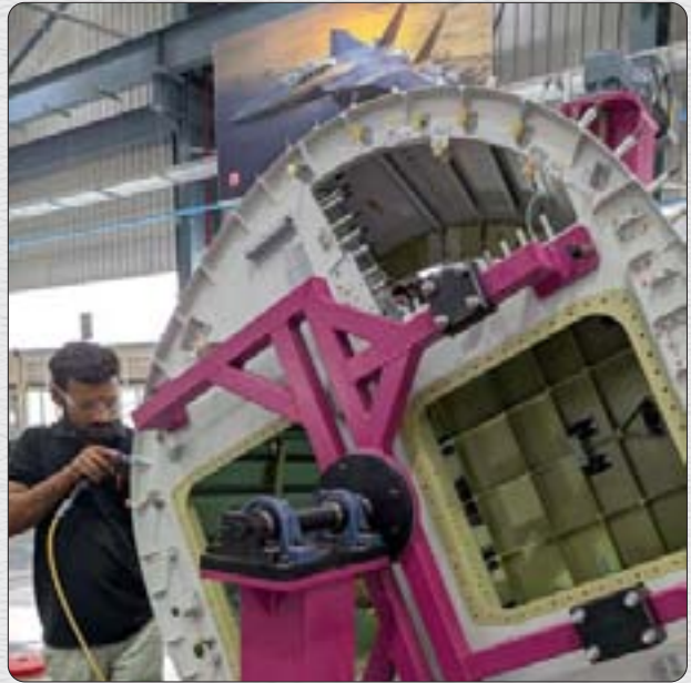
Dassault Falcon 6x Rear Fuel Tank Assembly Line
