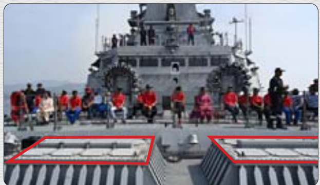
Vertical Launching Unit (VLU) structure (marked in red)
