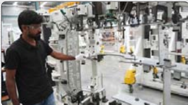
Industrialisation of A220 Door Jigs Laser Tracking & Calibration
