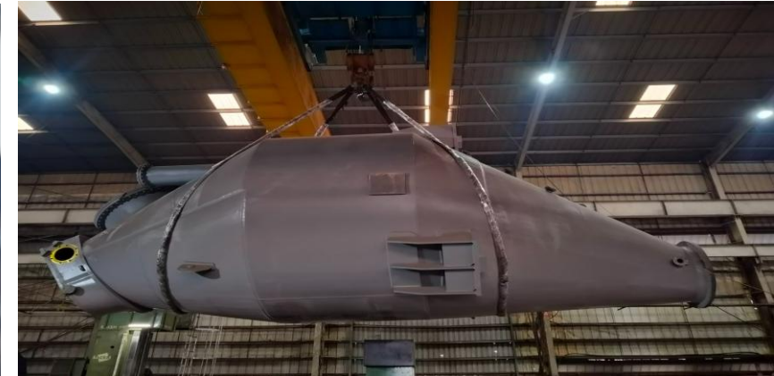
Material Hopper for Blast Furnaces
