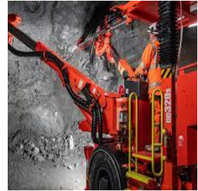
Twin Boom Jumbo Drill (8 Units)
