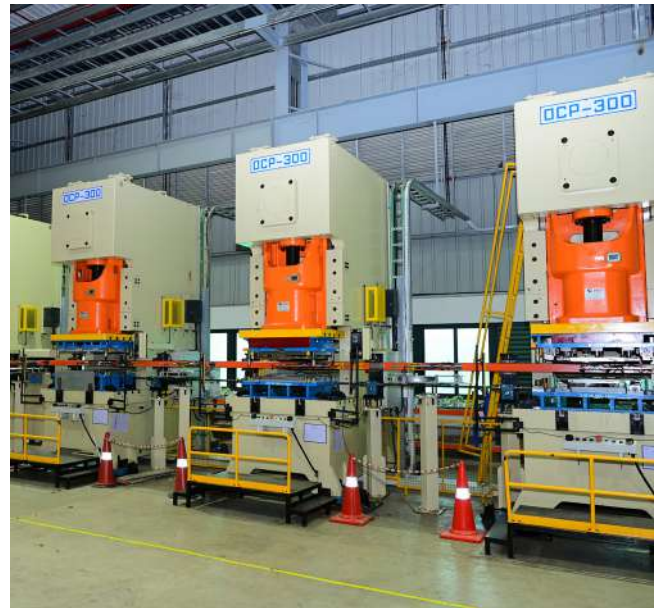
Tandem H Frame Press Machines in fabrication shop at Sri City Plant
